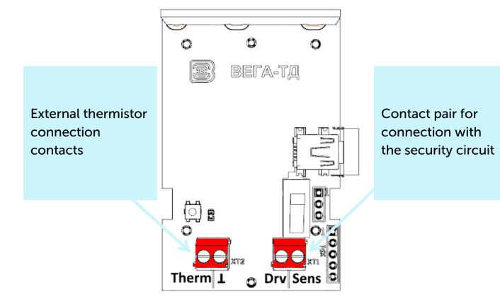
Temperature sensor has a two contact pairs. One pair ("Therm" and " $\perp$ " contacts) is for connect to external thermistor, another one is security input ("Drv" and "Sens" contacts).
