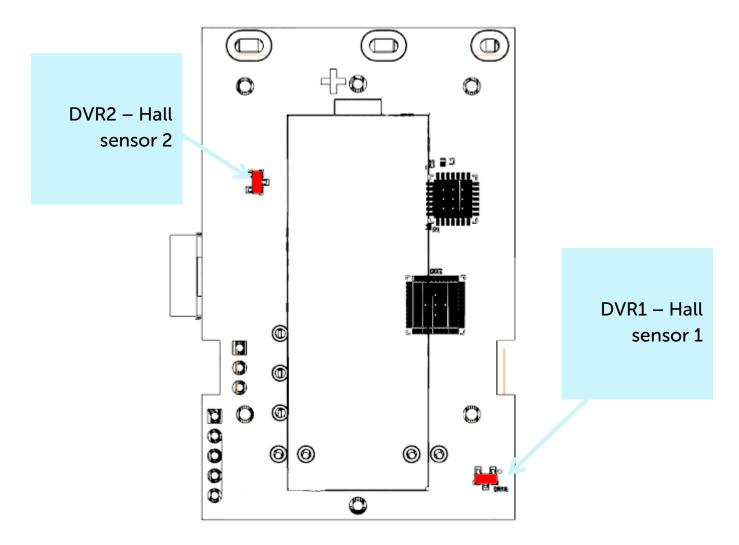
Tamper is located on the board top. Should the tamper triggering, the device sends a corresponding message to the LoRaWAN network.
